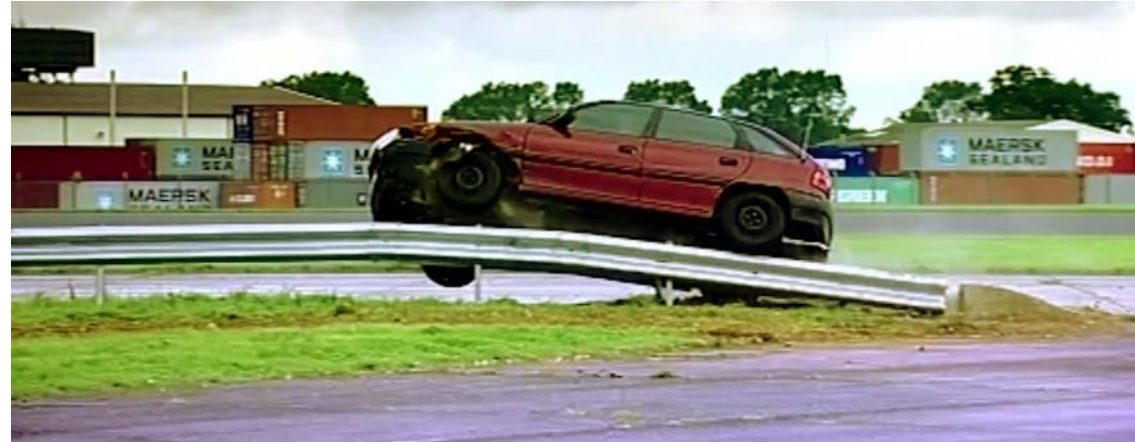
Full height and ramped down guardrail terminations present serious hazards even in low speed environments.
