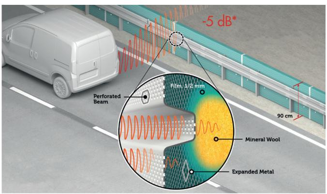
\*The noise reduction value has been determined by a specialized acoustic laboratory in accordance with ISO 9613-2.
